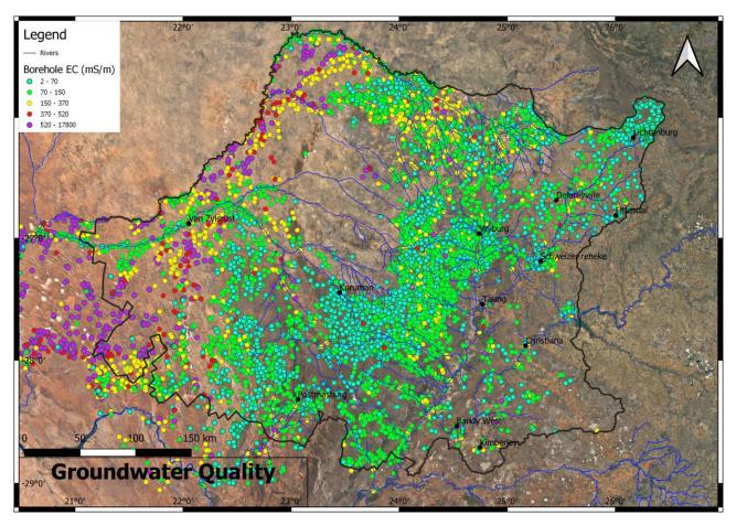
Figure 5-2 Borehole data for EC
